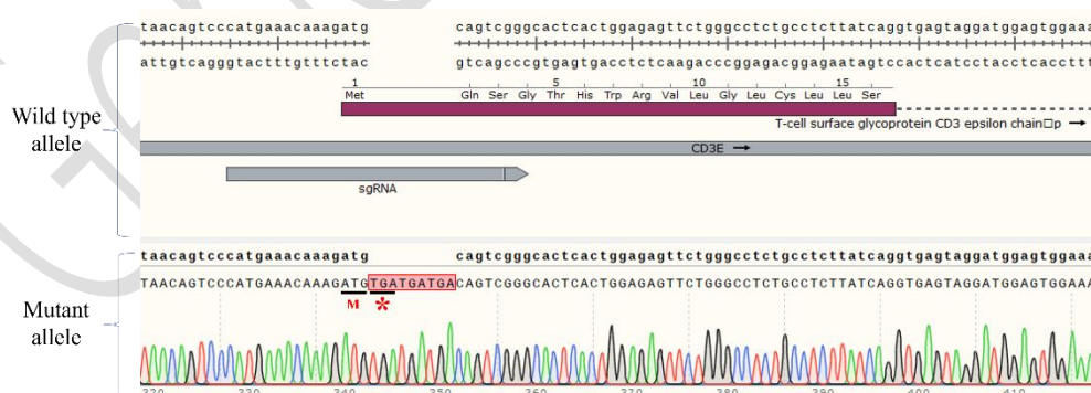
Figure 2 | The Sanger sequencing of the H_CD3E KO Jurkat Cell Line showed successful knockout of CD3E.
