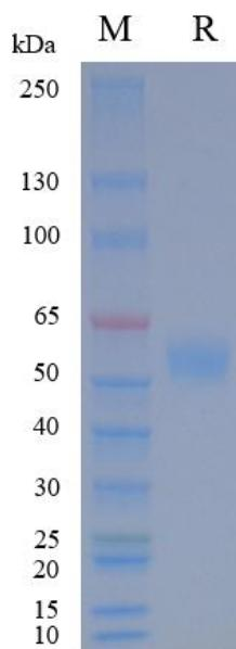
On SDS-PAGE under reducing (R) condition. The gel was stained overnight with Coomassie Blue. The purity of the protein is greater than 95%.
