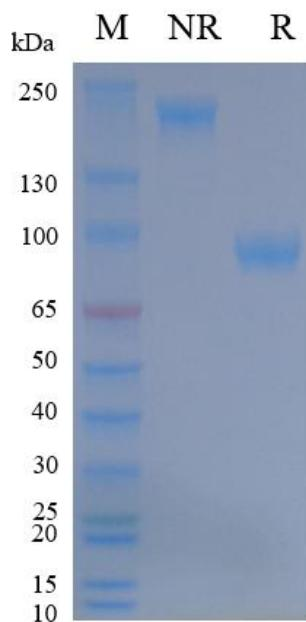
On SDS-PAGE under non-reducing (NR) condition and reducing (R) condition. The gel was stained overnight with Coomassie Blue. The purity of the protein is greater than 95%.
